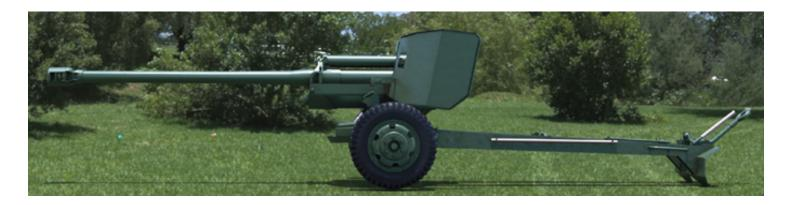
The modernized M56/15 variant with a barrel of 105-mm / 37 caliber. This new barrel has been evaluated for a life cycle of at least
